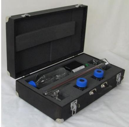
nZVI TESTER provides simple and fast measurement of zero-valent iron concentration in a product, even under the field conditions. The apparatus can be used for analysis of nZVI content in dry powder or slurry.
